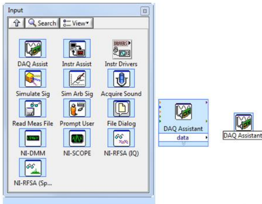
Figure 3. These are Express VIs as they appear on the palettes, an Express VI when first placed on the block diagram, and an Express VI when represented as an icon.
