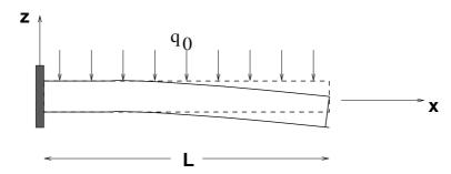
For a clamped cantilever aluminum beam the deflection function can be calculated by integrating the general differential equation for a beam and applying appropriate boundary conditions:
