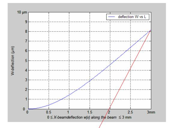
(d) Where is the maximum deflection, and how large is this deflection?  $\omega_{max}$  would be at the end of the beam and in the -Z direction
