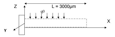
For a clamped cantilever silicon beam the deflection function can be calculated by integrating the general differential equation for a beam and applying appropriate boundary conditions:
