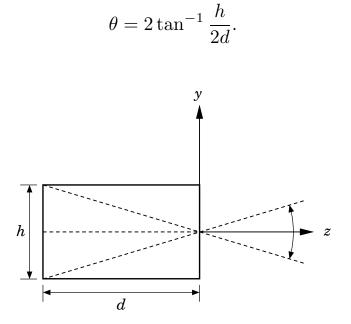
The pinhole camera has an infinite **depth of field**: every point in the field of view is in focus.
