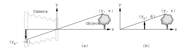
In the synthetic camera model we avoid the inversion by placing the film plane, called the **projection plane**, in front of the lens.
