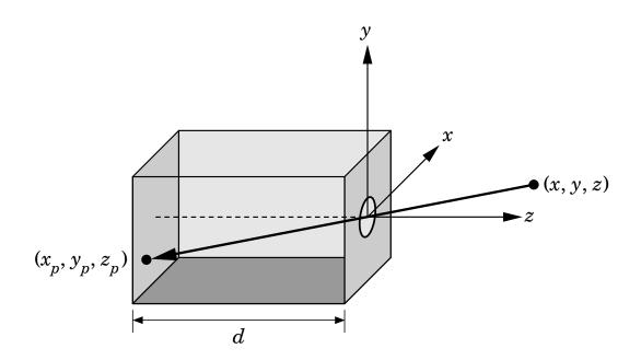
a box with a small hole in the centre of one side with the film placed at the other end. It is easy to model geometrically. Orient the camera along the z axis with the pinhole at the origin. Suppose the camera has length d. Assuming the pinhole allows only one ray of light from any point (x, y, z), the ray is clearly projected to the point  $(x_p, y_p, -d)$ , with coordinates
