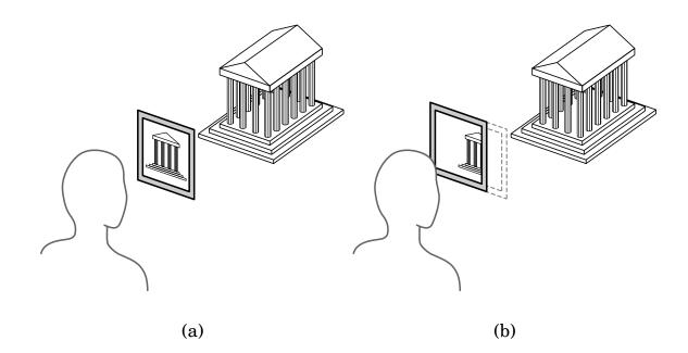
This is similar to the effect of the angle of view in a pinhole camera.
