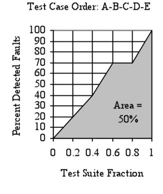
Let T be a test suite with n test cases and let F represent a set of m faults revealed by T. Let  $TF_i$  be the first test case in the ordering T' of T that reveals fault *i*. The APFD for the test suite T' is given by the following equation:
