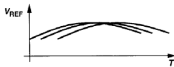
Figure 4 Output reference Vref vs. temperature.
