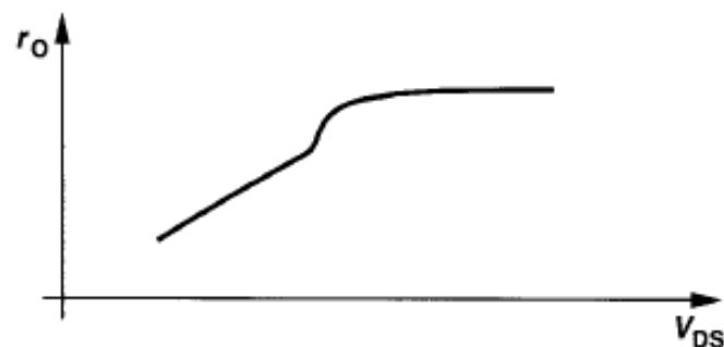
Figure 16.14 Kink in output resistance in Level 3 model.
