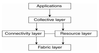
A layered architecture for grid computing systems.
