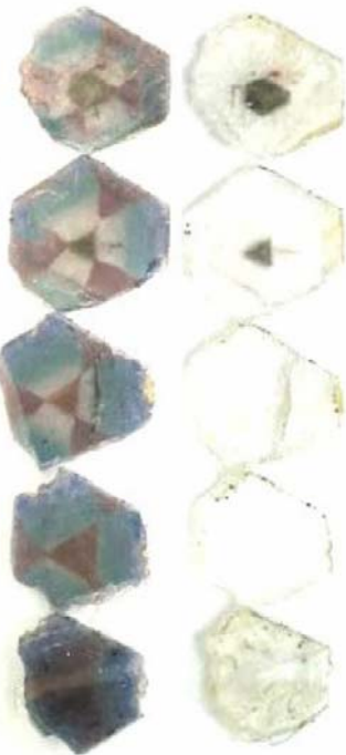
Figure 2. Slices of a single crystal of fluorite from Long Lake, New York. The top row is before irradiation, the bottom row is following irradiation.
