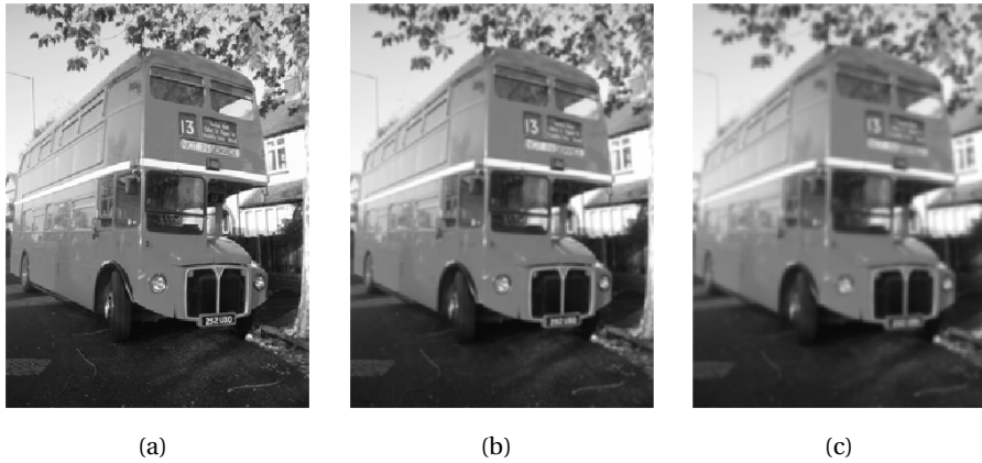
Figure 15.9. The images in (b) and (c) show the effect of smoothing the image in (a).
