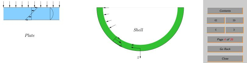
Some examples of constructions carrying loads using membrane stresses:
