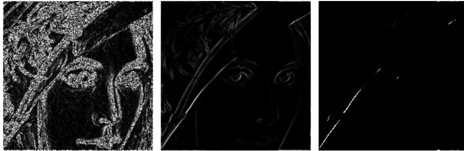
Figure 9.14: The computed gradient (left). In the middle the intensities have been normalised to the [0, 255] , and to the right the contrast has been increased.
