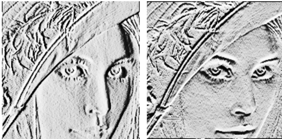
Figure 9.15: The first-order partial derivatives in the x - and y -direction, respectively. In both images, the computed numbers have been normalised and the contrast enhanced.
