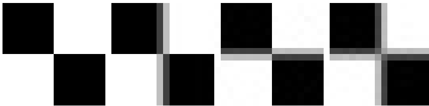
Figure 9.12: The results of smoothing the simple image to the left with the filter \frac{1}{4}\{1, 2, 1\} horizontally, vertically, and both, respectively.
