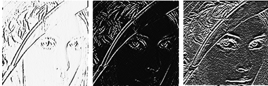
Figure 9.16: The second-order partial derivatives in the xx -, xy -, and yy -directions, respectively. In all images, the computed numbers have been normalised and the contrast enhanced.
