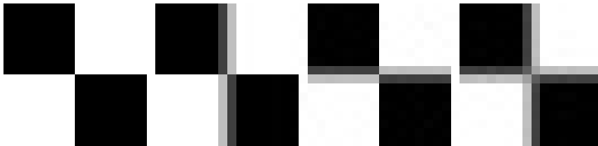
Figure 9.12: The results of smoothing the simple image to the left with the filter \frac{1}{4}\{1, \underline{2}, 1\} horizontally, vertically, and both, respectively.
