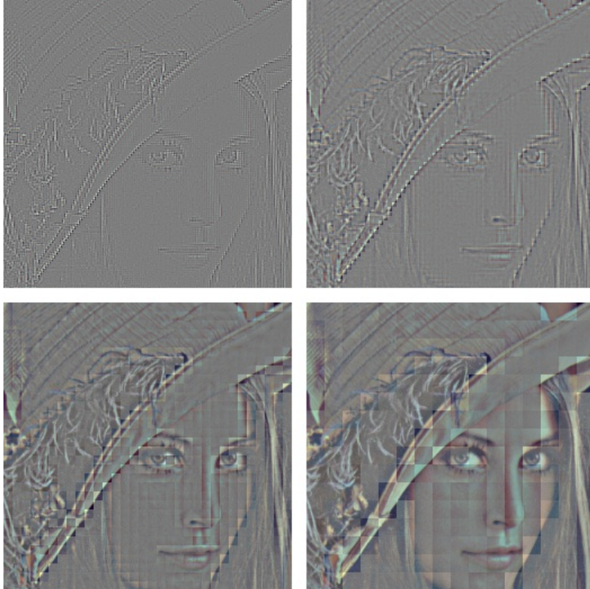
Figure 10.10: The corresponding detail for the images in Figure 10.9, with the Haar wavelet.
