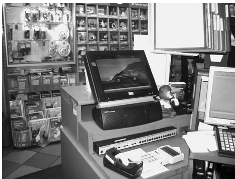
Figure 9.2 First prototype (touch screen) created by the IT department based on the mock-ups created in the design workshop. It is located next to the cash register, facing the attendant
