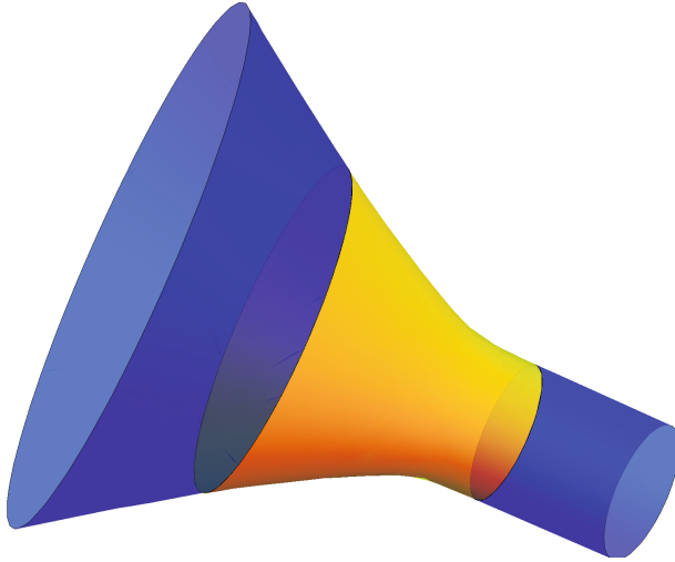
Fig. 6. Implicit blending surface (yellow) between cone and cylinder (blue) from Example 3
