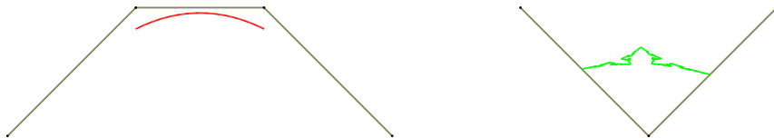
Fig. 6. Left: a cubic spline with 4 control points. Right: a fractal curve with 3 control points.
