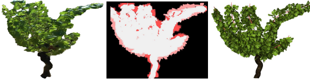
Fig. 10. At the left, the original image. At the right, the reprojected model. In the middle, the projection errors map. White pixels correspond to pixels where the original image and the reprojected one are superposed and red pixels are wrong pixels.
