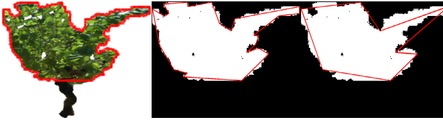
Fig. 5. DCE algorithm examples. At the left, the original image with the contour points around the foliage. The two other images show the DCE algorithm with a 24-point polygon in the middle and a 8-point polygon on the right. The inward angles are represented in blue.
