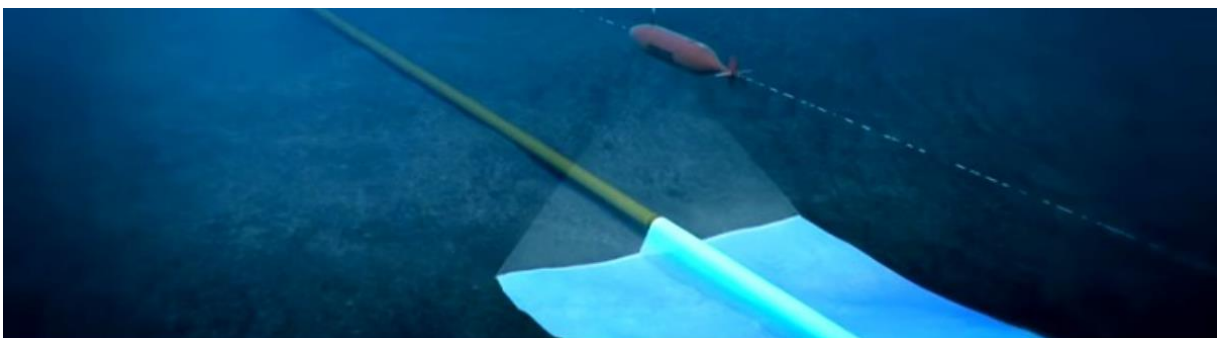
Figure 1: Hugin AUV inspecting an underwater pipeline (source: Kongsberg Maritime)
