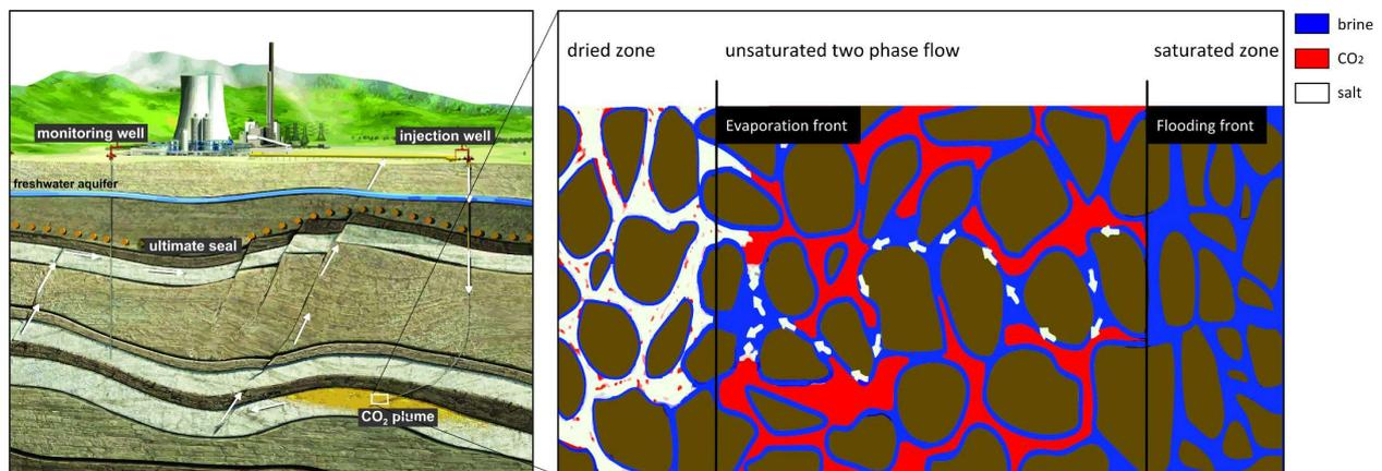
**Figure 1.** Potential zones and fluid-solid phases in the near-well environment during CO<sub>2</sub> injection in saline aquifers.
