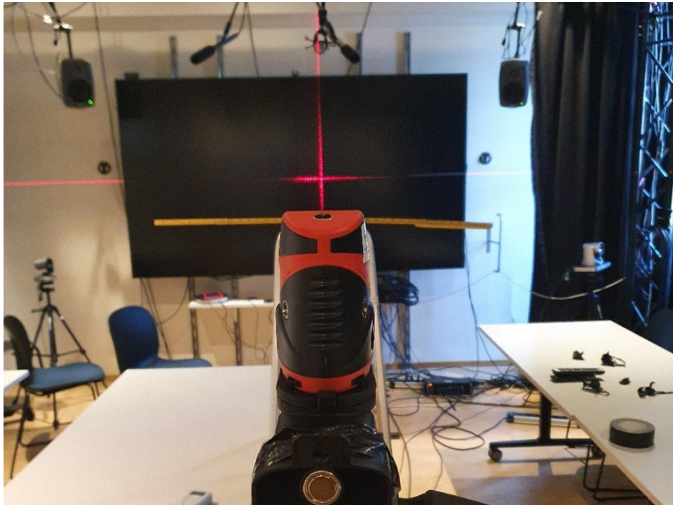
Figure E.3: Alignment of the centre of the measure, the laser pointer attached to the pendulum, and the laser point on the screen.
