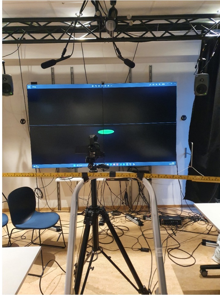
Figure E.2: The measure below the pendulum. The black bars signify the centre of the measure and \pm 10 cm
