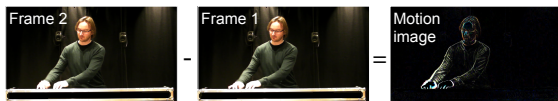
Figure 1.3: A motion image is created by subtracting subsequent frames in a video file (Frame(2) - Frame(1)).
