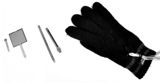
Figure 1.9: Examples of small and large force and bend sensors (left) and a custom-built glove with similar sensors built-in (right).
