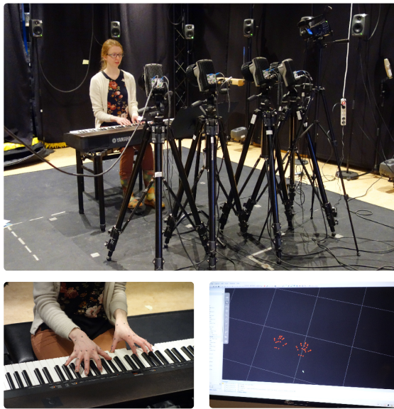
Figure 1.8: Setup for motion capture of pianist Christina Kobb. In addition to the cameras placed in front, there are also cameras placed behind the pianist to capture the motion in three dimensions.
