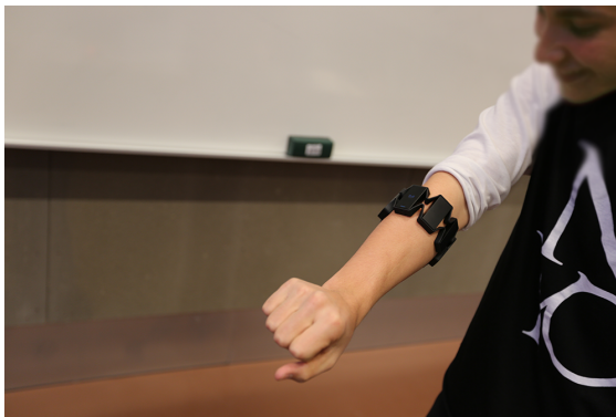
Figure 1.13: An example of music interaction with the commercially available MYO armband, which contains eight EMG sensors, accelerometers and gyroscopes (Photo: Kristian Nymoén).
