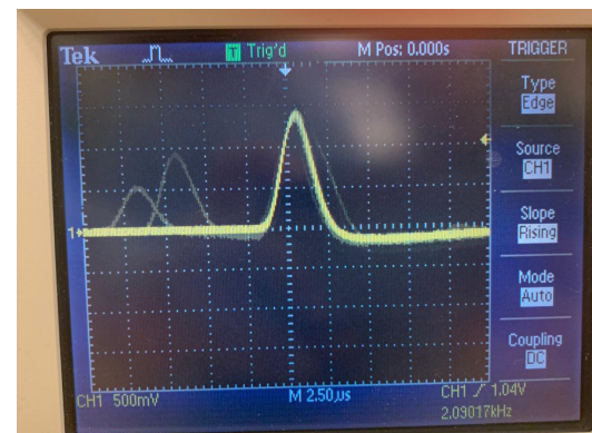
Figure 17.8 Intercomparison of typical pulses at sequential points along the signal processing chain.
