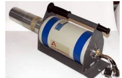
Ge detector + dewar filled with a liquid nitrogen
