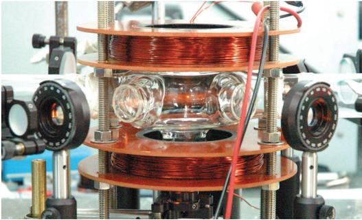
**Figure 11.30:** Illustration of a MOT. The atoms are “collected” in the center of the glass container. A laser enters from the sides, while a magnetic field is generated by the coils.
