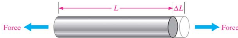
(a) Strain occurs as length changes from L to L + \Delta L when force is applied.
