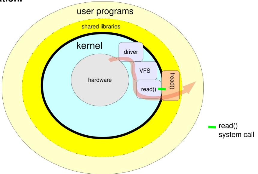
Data is transferred from the hardware via a driver and VFS (virtual files in the kernel, when the user-program calls fread() (standard C-library fu
