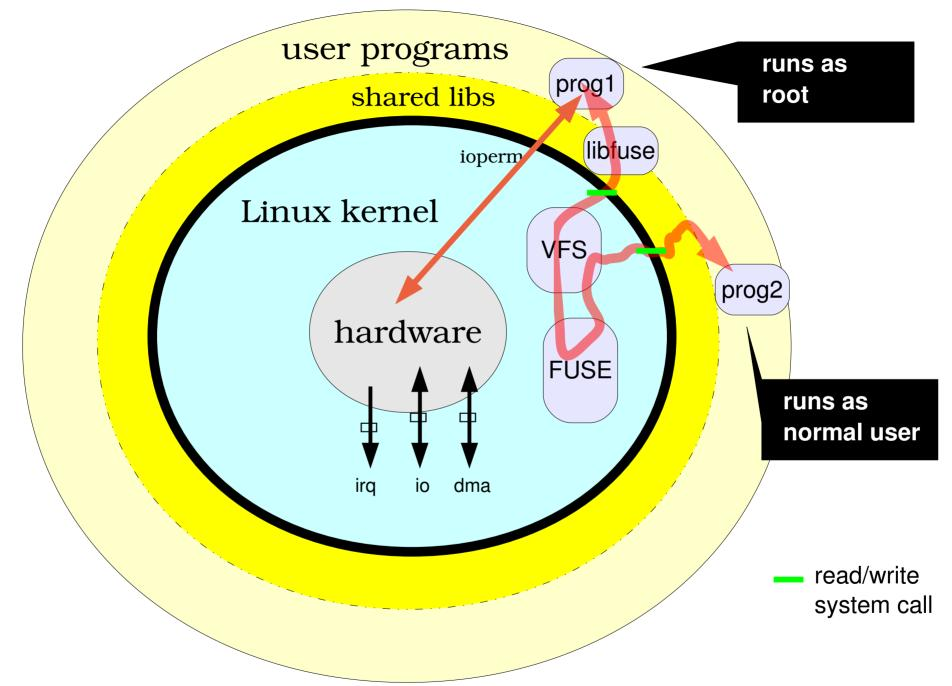
FUSE allows the driver to be implemented as a root-program in userspace while the main application program is run as a normal user.
