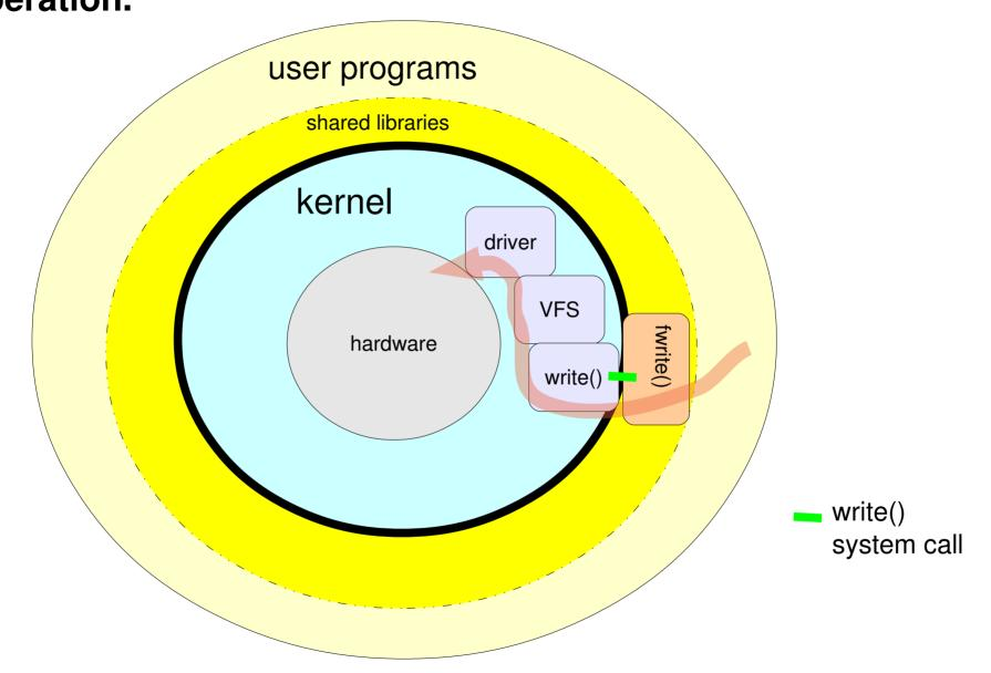
Data is transferred to the hardware via the driver and VFS in the kernel, when the user-program calls fwrite() (standard C-library function-call).
