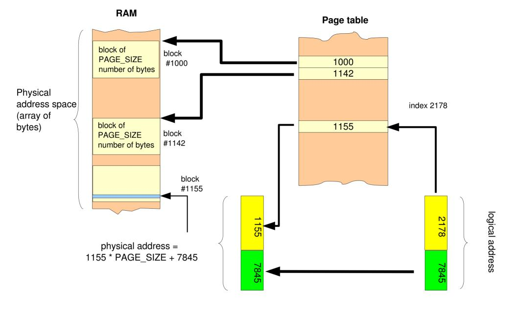
Principle of memory mapping. CPU-instructions use *logical* addresses. The CPU looks these up in a table to obtain the *physical* address to use on the address bus.
