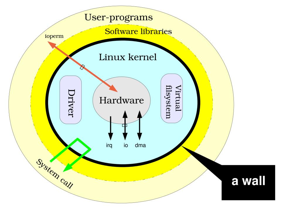
Shell model. Protected mode. User programs have to use system calls to gain access to the kernel. Only the kernel has access to the hardware. One exception is the use of ioperm().
