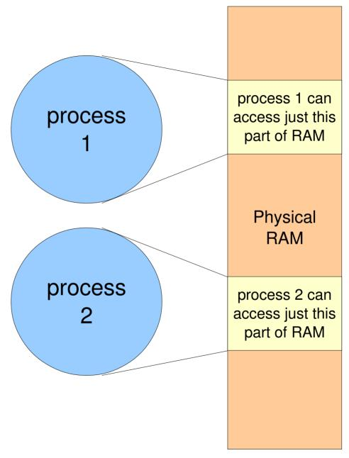
Simple example: Two processes each have been assigned one region of the physical RAM
