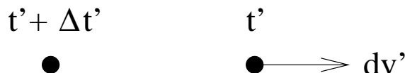
Figure 3.5: In RF two points on the circumference are accelerated at different times. Thus the distance between them is increased.
