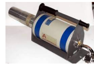
germanium detector + dewar filled with a liquid hydrogen
