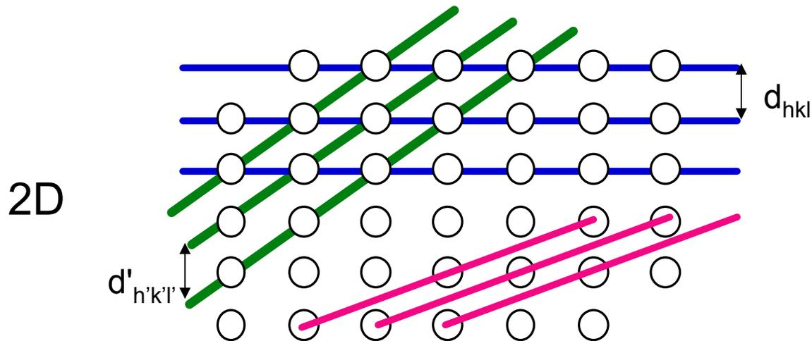
Inter-planar spacings can be measured by x-ray diffraction (Bragg's Law)
