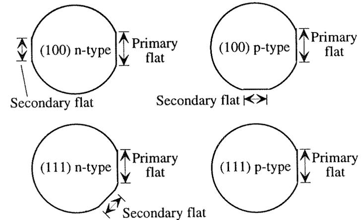
Primary and secondary wafer flats are used to identify orientation and type.
