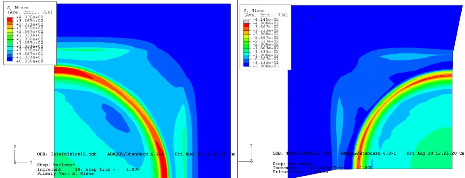
Stress distribution caused by: Left 1 bar pressure from the top, top view. Right 1 bar pressure from the bottom, bottom view. Only  $\frac{1}{4}$  of the membrane is simulated. The stress shown is the von Mises stress in MPa.
