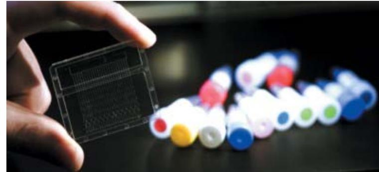
Measuring flow rates of enzymes into bacteria analysis chip
