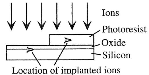
Figure 3.7. Illustrating the use of a photoresist mask to keep the implant from reaching the silicon in selected regions.
