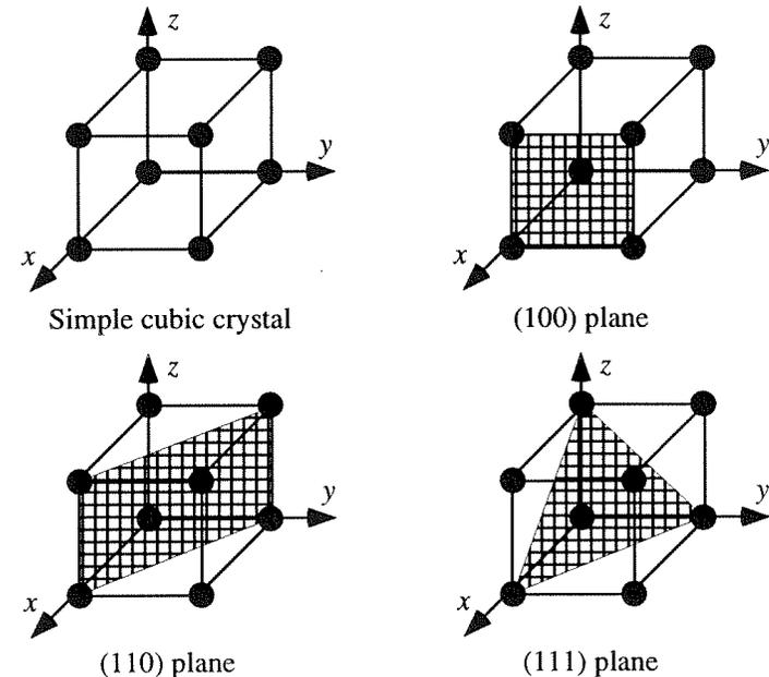
re 3.1. Illustrating the different major crystal planes for a simple cubic lattice of atoms.
