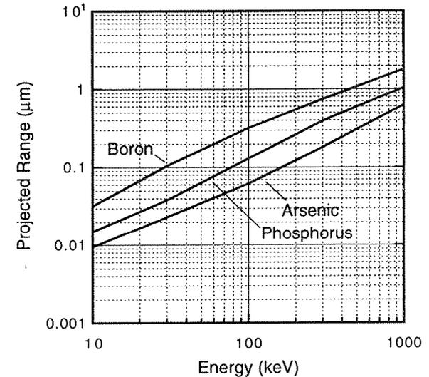
Figure 3.6. Projected ranges of ions implanted into silicon ( redrawn from [7]).
