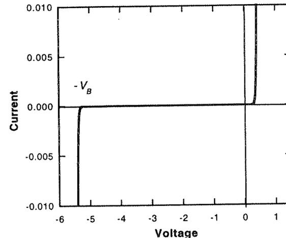
Figure 14.3. A typical diode current-voltage characteristic.
