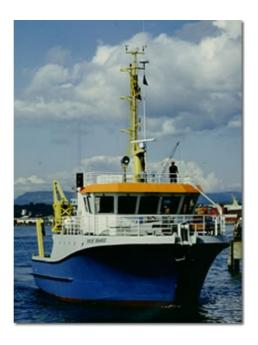
F/F Trygve Braarud is the biggest sea-going vessel of UiO. It is a floating laboratory with modern sensors for measuring physical, chemical and biological parameters. Its normal region of operation is the inner and outer Oslo fjord. F/F Trygve Braarud, built in aluminum, was constructed in 1983 at Linstøls Skips- og Båtbyggeri in Risør, Norway. The vessel is 21.8 meters long, has a normal cruising speed of 9.5 knots (18 km/h) and a maximum speed of 12 knots (22 km/h).
