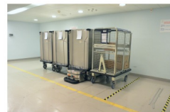
Figure 2: AGV placing the cart in a niche
