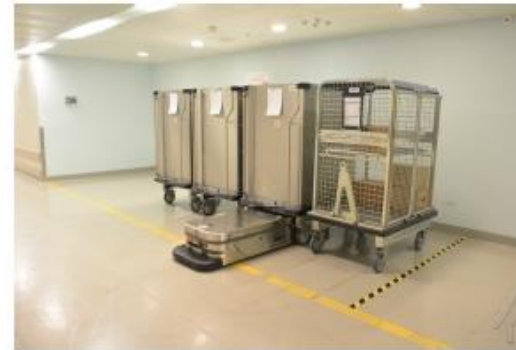
Fig. 2. An AGV picking up a cart
