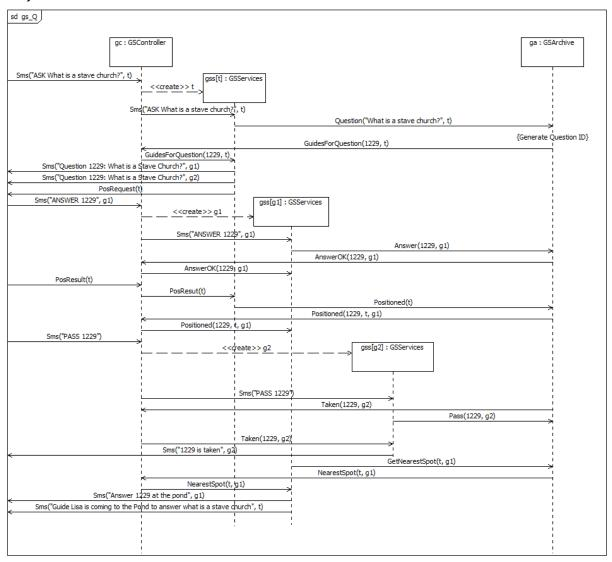
Remarks: last parameter in signals is always the routing parameter (identifier). Lifelines that explicitly end within the Interaction are *destroyed/terminated*.
