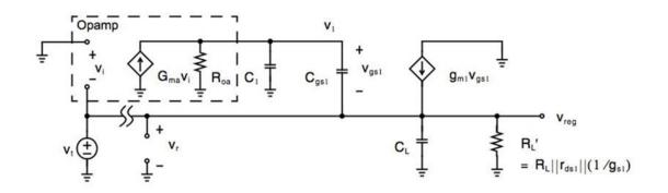
$$L(S) = \left(\frac{G_{m_A} R_{o_A} R_L}{R_L + \frac{1}{g_{m_I}}}\right) \frac{\left(1 + \frac{S}{w_z}\right)}{\left(1 + \frac{S}{w_{p_I}}\right)\left(1 + \frac{S}{w_{p_I}}\right)}$$
