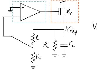
$$V_{reg} = V_{ref} \left( 1 + \frac{R_1}{R_2} \right)$$
