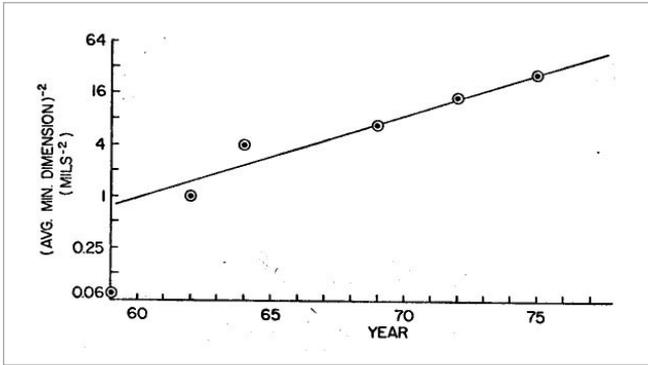
the average of the two is a good parameter to relate to the area that a structure might occupy. Density can be expected to be proportional to the reciprocal of area, so the contribution to improve density vs. time from the use of smaller dimensions is plotted in Figure 3.
