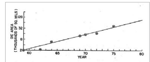
Density was increased partially by using finer scale microstructures. The first integrated circuits of 1961 used line widths of 1 mil (~25 micrometers) while the 1975 device uses 5 micrometer lines. Both line width and spacing between lines are equally important in improving density. Since they have not always been equal,
