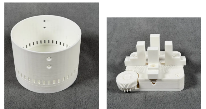
Early motor-holder concepts: cylinder design and heavier 4-jaw chuck.
