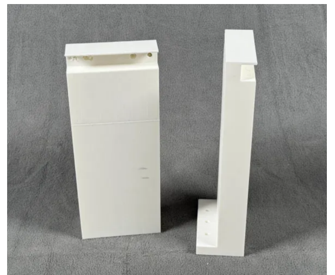
First load-cell holder that blocked sensor bending; later re-designed.
