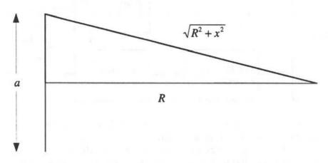
The differential path length  $\Delta$  associated with a point x on the aperture and a range R can be evaluated using simple geometry.
