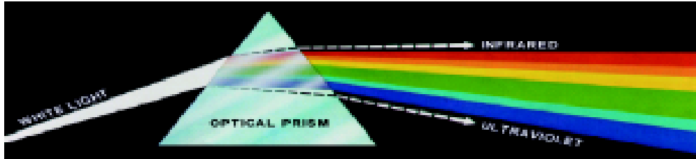
Figure 2-22. A qualitative illustration of chromatic refraction through a prism.
