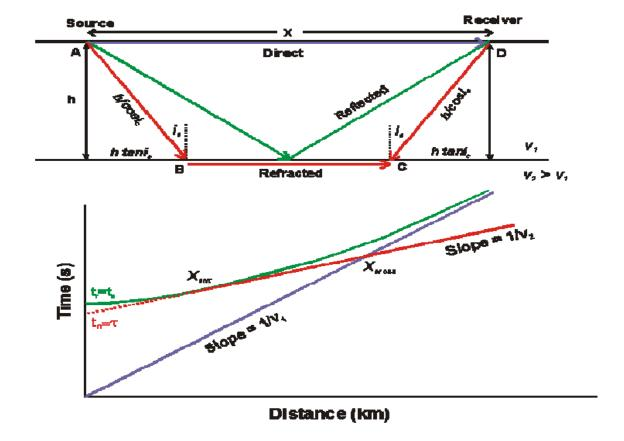
We consider a simple two-layer model as shown in the figure above, where the P-wave velocity of layer l and l is  $v_l$  and  $v_l$ , respectively (note  $v_l > v_l$ ). In general, a receiver will measure three different wave contributions: direct wave, reflected wave and refracted wave.
