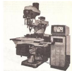
FIGURE 1.8. NC system operating machine tool and controller. (Courtesy of Bodgopt Industrial Division of Tacton Inc.)
