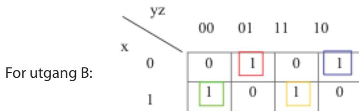
For utgang B =  $x'y'z + x'yz' + xy'z' + xyz = x'(y'z + yz') + x(y'z' + yz)$
