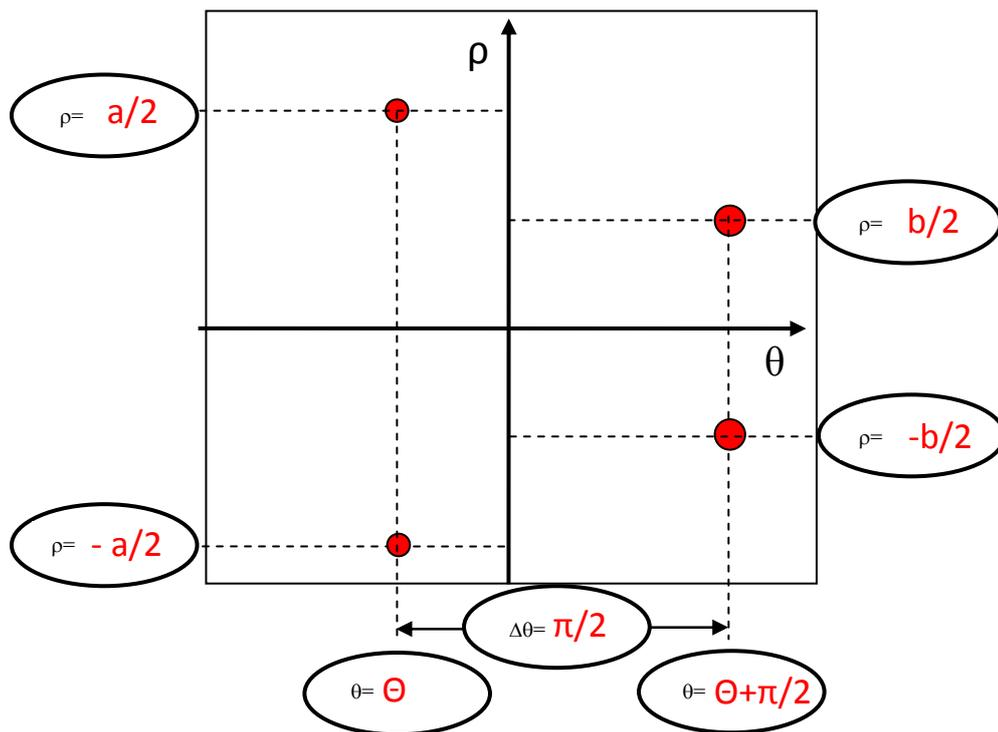
There are four line segments in the image, making a rectangle with sides  $a$  and  $b$  ( $a > b$ ). So there will be four peaks in Hough space, with different heights, indicated by different sizes of the red dots. The sides of length  $a$  (large dots) are at a distance  $b/2$ , while the sides of length  $b$  are at a distance  $a/2$  from the origin.
