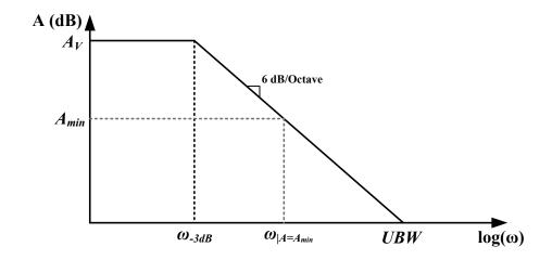
For a single-pole system, when  $\omega > \omega_{-3dB}$ , it is defined that A decreases 6dB/octave (which is not 100% true, see the appendix). This means A decreases by two when  $\omega$  increases by two and GBW is a constant when  $\omega > \omega_{-3dB}$ .
