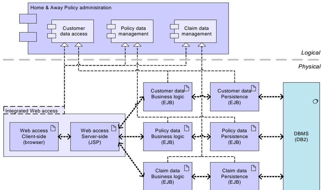
Figure 16. Mapping of logical application components of the ArchiSurance policy administration onto physical artifacts.
