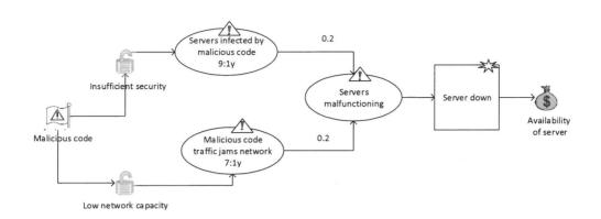
b) If the diagram is complete, then there are no external threat, and we can calculate the frequency of the threat scenario Servers malfunctioning with the help of the other two threats: Servers infected by malicious code and Malicious code traffic jams network.
