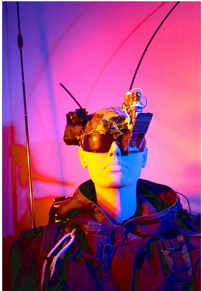
Figure 3: An early to mid 1980s eyeglass-based lifelogging and computer mediated reality system, recently shown at the Smithsonian Institute, National Museum of American History, as well as at SIGGRAPH. This system was developed for the production of visual art in a computer mediated reality environment. The picture itself was captured using another similar system, and similar methodology.
