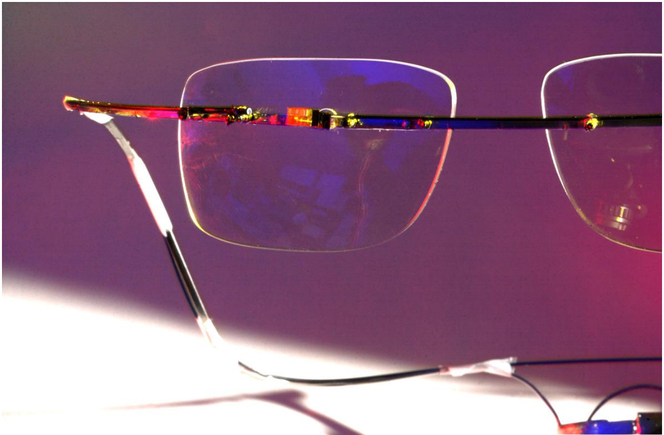
Figure 4: Eyeglasses having illusory transparent frames. When worn, the frames pass directly over the eyes, and the wearer sees “through” the frames by way of computer controlled laser light that resynthesizes rays of eyeward bound light. This fully functional but crude prototype leaves the workings visible, but in actual manufacture, the workings may be completely concealed within the frames.
