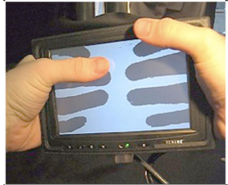
LucidTouch enhances back-of-device interaction by visualizing the user's hand position.
