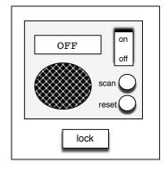
Below is a proposed state machine of this model, which uses the alphabet {on, off, scan, reset, lock}. Here we ignore the current frequency and scanning is done by pressing scan repeatedly until the lock button is pressed.
