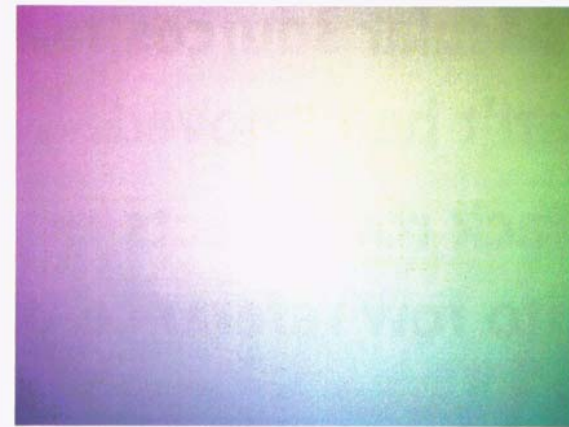
Color shading: color planes have different centers (because of pixel asymmetry)
