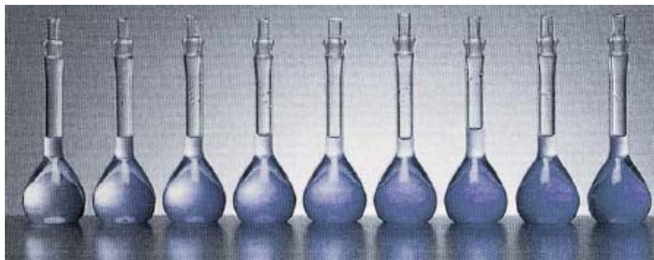
Figure 1: Standard solutions with blue phosphate molybdate complex.
